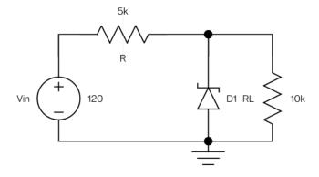
the input voltage is 120 V and voltage across Zener diode is 50 V, calculate:
